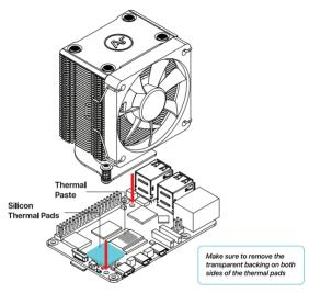
2. Affix screw at the bottom of the mounting pins to fix the Argon THRML 60 Radiator Cooler.
