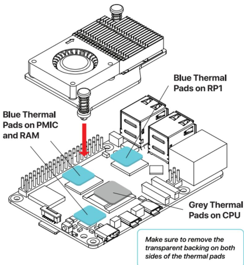
2. Push mounting pins to fix the Argon THRML 30 Active Cooler.
