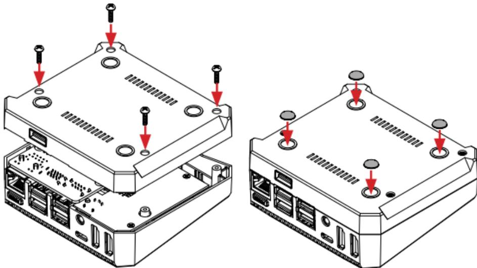
Use longer **round head screws** to fasten bottom cover and place **rubber footings**.
