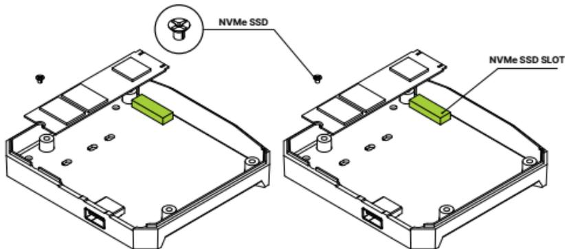
Secure your **NVMe Drive** to the **Argon ONE NVMe Expansion Board**. You may move the screw point on the Board to the appropriate size of your Storage Drive.
