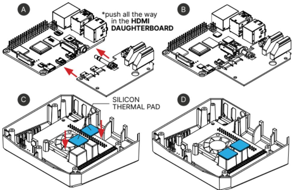
Reminder: Peel off plastic on both sides of the thermal pad
